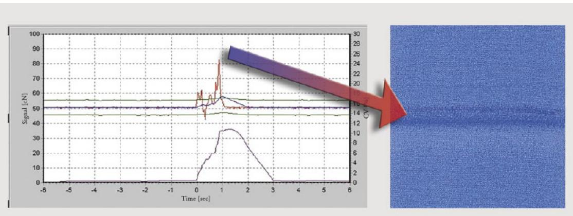
The most important quality parameter in texturing is the correct yarn tension. Abnormal tension levels and peaks result in dyeing problems.
